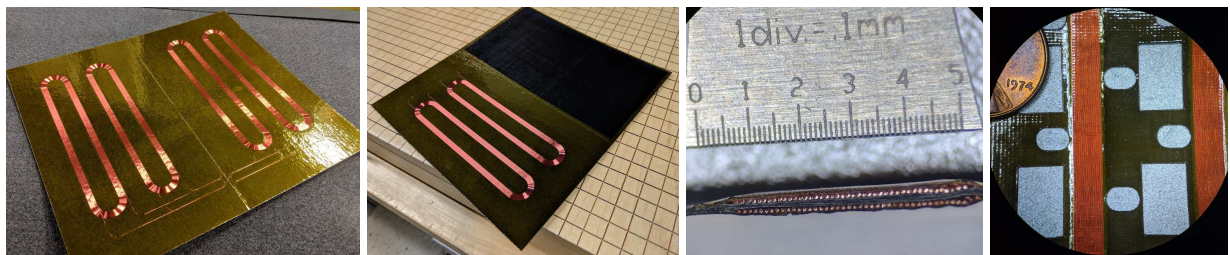
Figure 6.16: Wire plotting the planar coils for the Lorentz force actuator to drive traveling waves. a) Mirror images of the 25 turn coils are plotted and cut out, b) The plotted sections are folded around a piece of carbon prepreg and cured, c) A microscope section view of the double layered planar coils. d) Microscope image of cured planar coil, with additional features cut (U.S. penny coin for scale).
