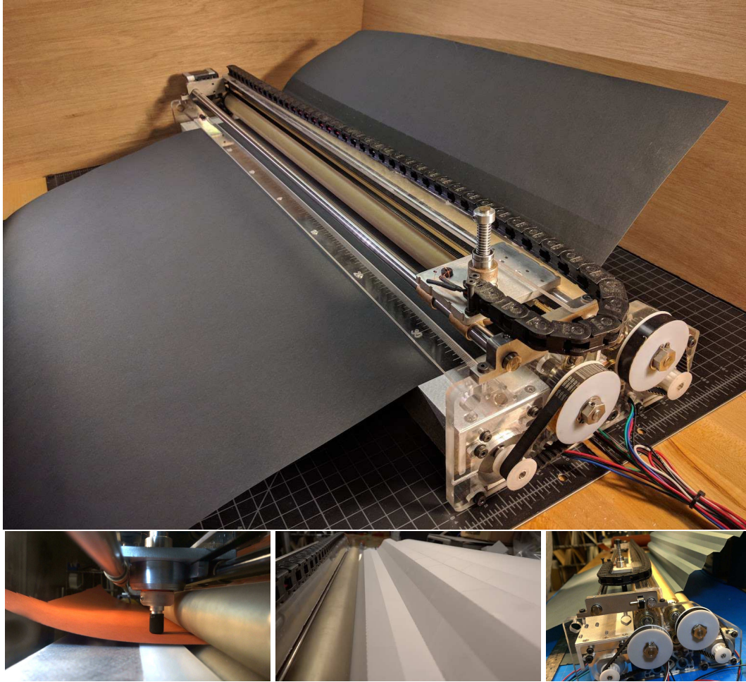
Figure 2.7: a) Machine for cutting and folding used in processing shaped honeycombs. b) Voice coil drag knife cutting stage, c) Cut and folded output from machine, d) Machine processing vulcanized fiber.
