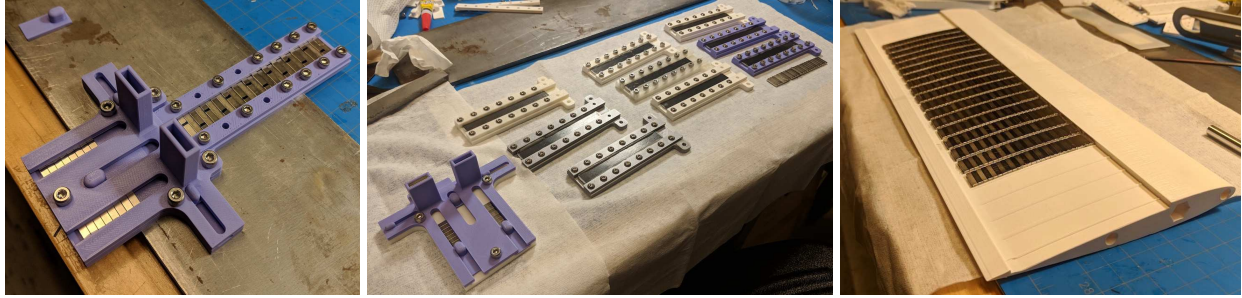
Figure 6.23: Halbach assembly aids. a) Halbach extruder draws from four cartridges of magnets, one for each orientation, b) Cartridges are filled and bonded to a thin piece of carbon, c) Halbach arrays are transferred to the hydrofoil.
