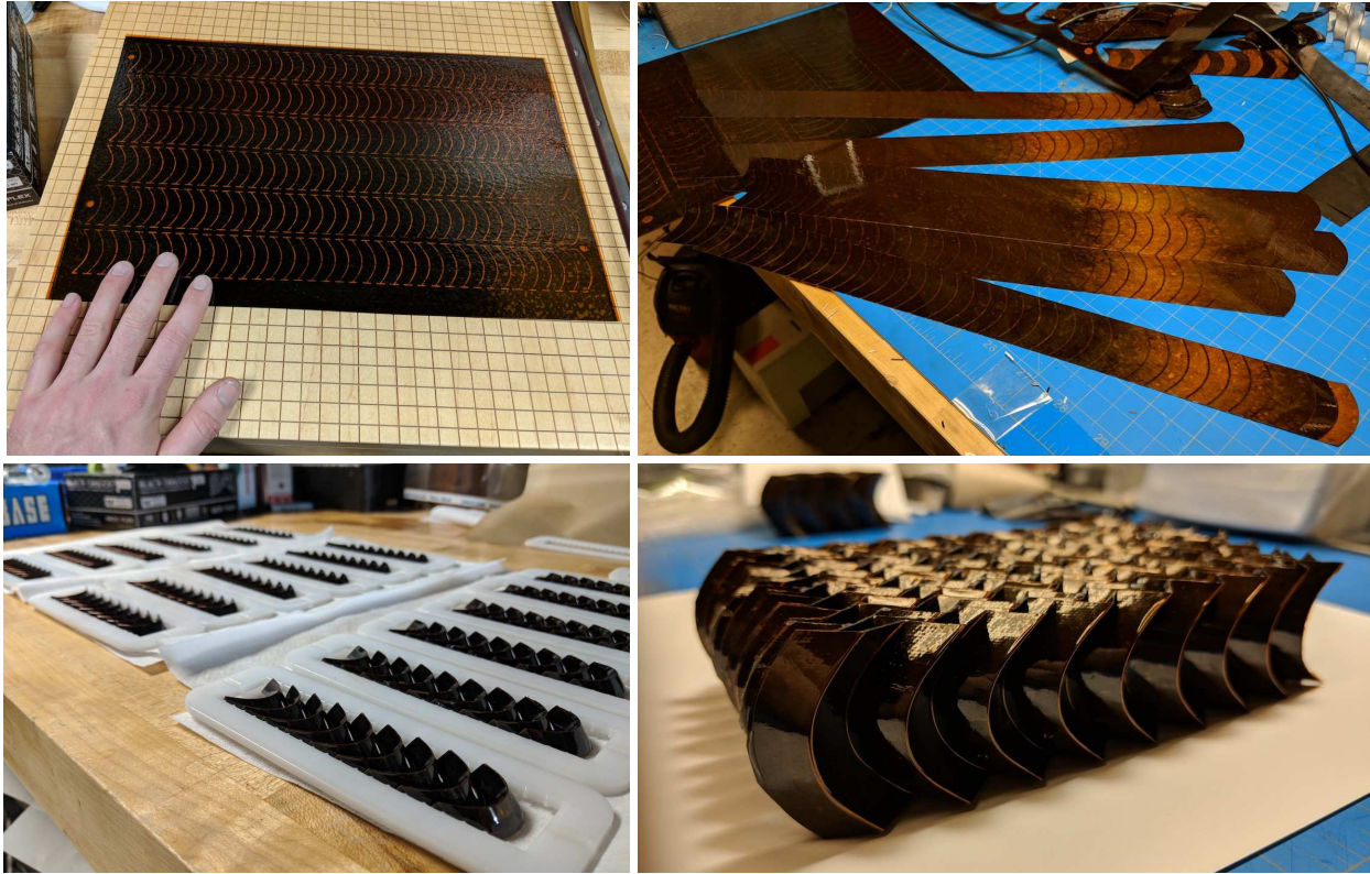
Figure 4.11: Making carbon-polymer curved crease architected materials a) Cured laminate with patterned hinges, b) Laminate cut into strips, c) Strips folded in frames, d) Strips assembled and bonded into volume.
