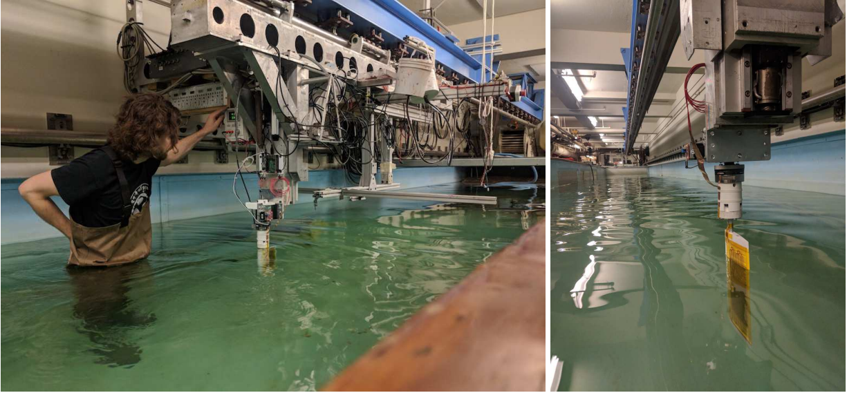
Figure 6.28: Tow tank testing setup. a) The author installing traveling wave experiment on tow tank carriage. b) View down the tow tank with water level lowered, showing loadcell, collet-holder, and traveling wave prototype.
