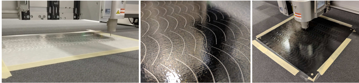
Figure 4.9: a) Cutting prepreg with an oscillating knife to form hinge lines, b) Cured prepreg between polymer sheets, c) Optically registering and cutting of additional features in the cured laminate
