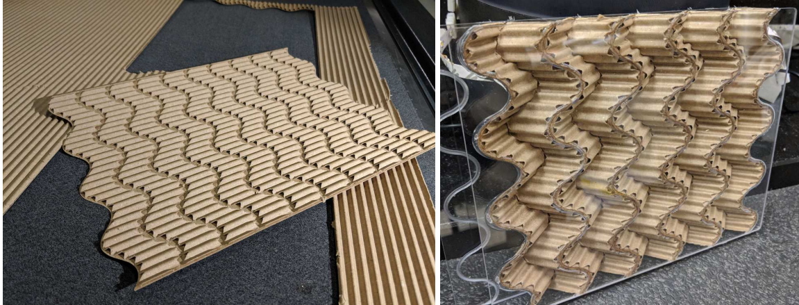
Figure 5.9: Corrugated curved crease foldcore prototypes in cardboard. a) Flat pattern after cutting crease curves from the corrugated layer, b) Folded and sandwiched between polycarbonate plates.
