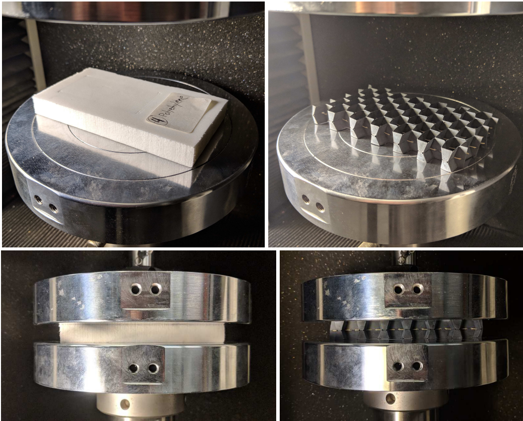
Figure 3.6: A) Foam sample on test platen, B) Folded sample on test platen, C) Foam sample loaded by platens, D) Folded sample loaded by platens.
