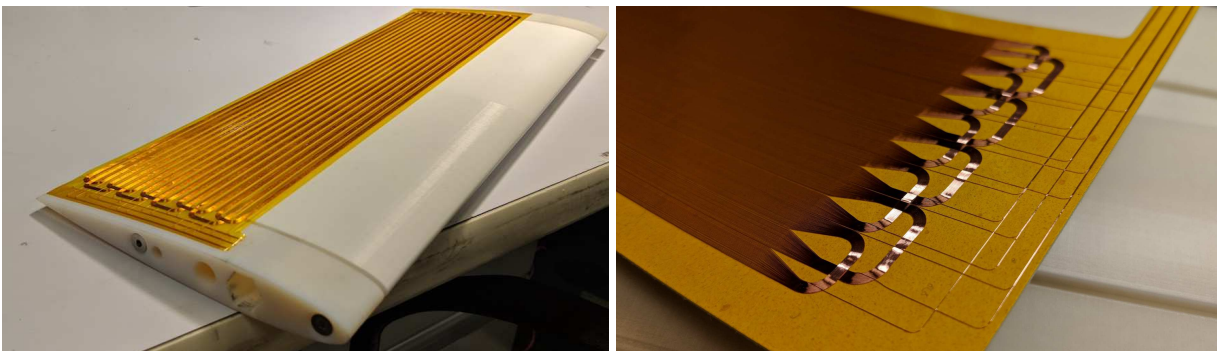
Figure 6.20: a) Actuated membrane applied to NACA12 hydrofoil, b) Lead connections for three-phase actuation.
