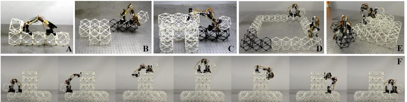
Figure 13: Robot experiments. A) 1D beam reconfiguration, B) 2D plate assembly, C) 3D enclosure assembly, D) Multi-robot construction of branching structure showing global precision from part metrology, E) Multi-robot construction of 35 voxel pyramid, F) 3D locomotion and voxel transport.
