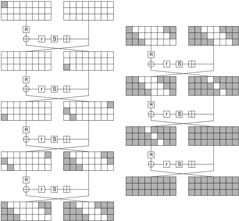
**Fig. 2.** Diffusion process: grey boxes represent active bits
