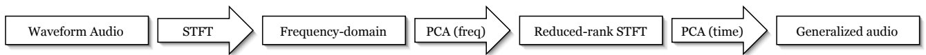
Figure 2: General overview of our synthesis by analysis system. Time domain audio is converted to the frequency domain and then rank-reduced to a low number of frequency dimensions. Multiple short time chunks of these frequency fingerprints are then lined up and given to another PCA algorithm, which reduces dimensionality along the time axis. The end result is a spectral fingerprint representing “generalized audio,” or the observational mean of the audio perception. This resultant data is invertible back to the time domain via inverting both the time and frequency PCA weight matrices. Enhancements to this process (described below) include adaptive dimensionality reduction (for a real-time effect implementation) and beat and tempo locking for synthesis of a generalized texture loop.
